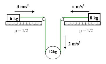
Find the acceleration of the 8 kg mass. The coefficient of friction at both tables is 1/2
